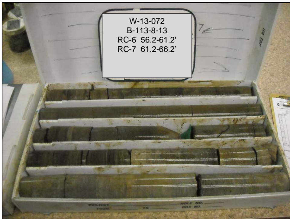
B-113-8-13 – RC-6 and RC-7 – Depth from 56.2 to 66.2 feet
